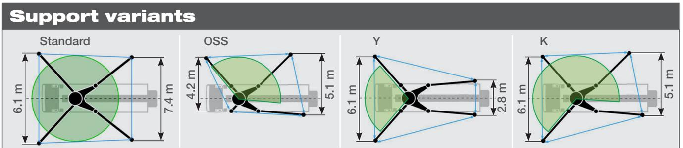
Boom delivery line max. 85 bar. All data max. theor. Support width based on center of support leg. OSS and K left and right possible
