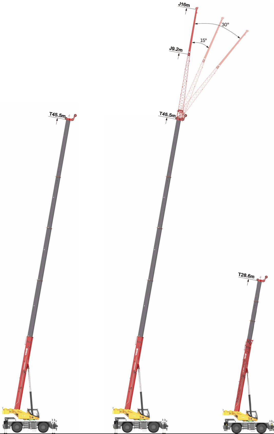
Telescopic boom on outriggers 主臂、支腿吊载
