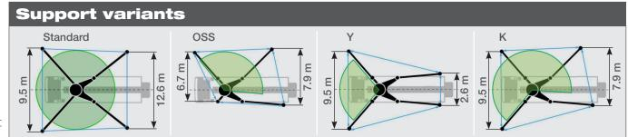
Boom delivery line max. 85 bar. All data max. theor. Support width based on center of support leg. OSS and K left and right possible
