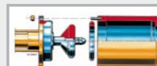
Simple valve change without removing the pipeline
